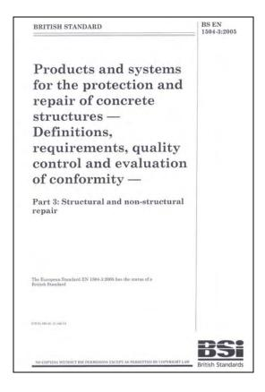
BS EN 1504-3 provides performance characteristics and requirements for structural and non-structural repair products under the following 3 repair principles.
