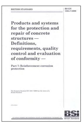
BS EN 1504-7 provides requirements for the protection of <u>existing</u> uncoated steel reinforcement and embedded steel in concrete structures under repair.
